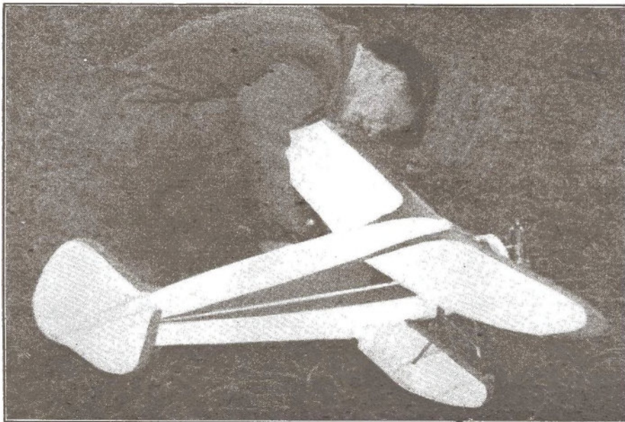
Morris Mountjoy, of Hyattsville, Md., fastens the lock pins to hold the wings of his Brown-powered Waco. Wing panels are designed to shear off upon impact without injuring rest of the structure.
